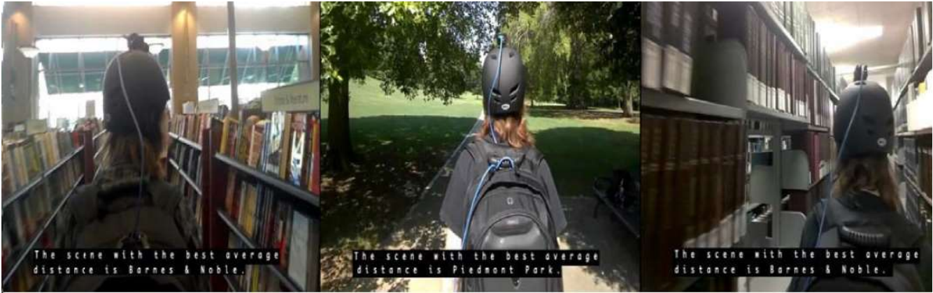
Figure 2 A helmet-worn prototype is used to match the scene that the student is currently encountering to a set of stored scenes. For this prototype the system then stated the scene’s label to the user. For the proposed system, the scene will be matched to predefined privacy settings.
